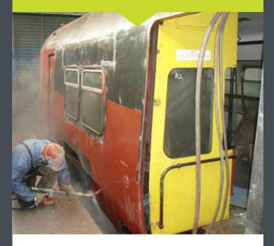
Stripping paint and corrosion is a common requirement when it comes to things transport. Water jetting is a much better option for stripping paint and corrosion from around vulnerable items.
